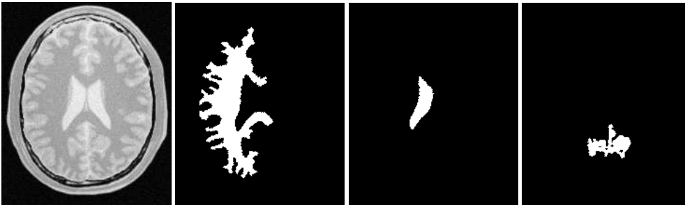
Figure 9.26: Images generated by the segmentation process based on the ThresholdSegmentationLevelSetImageFilter . From left to right: segmentation of the left ventricle, segmentation of the right ventricle, segmentation of the white matter, attempt of segmentation of the gray matter. The parameters used in this segmentations are presented in Table 9.6
