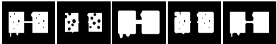
Figure 11.10: The effects of morphological operations on a binary image using a circular structuring element of size 4. From left to right are the original image, erosion, dilation, opening, and closing. The opening operation is erosion of the image followed by dilation. Closing is dilation of the image followed by erosion.
