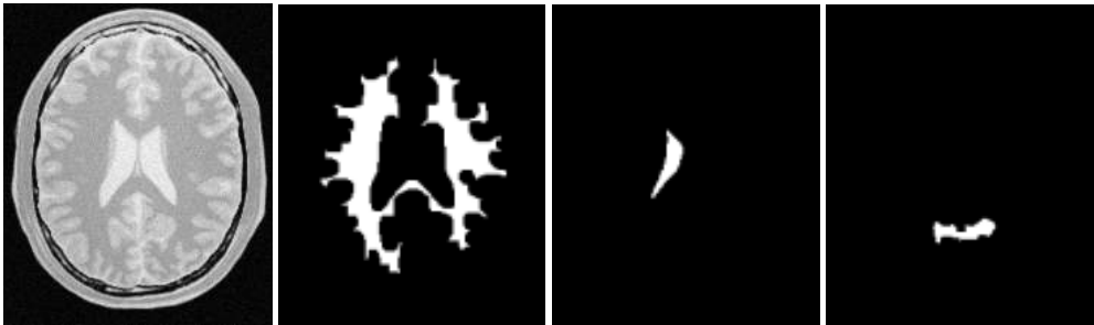
Figure 9.3: Segmentation results of the NeighborhoodConnectedImageFilter for various seed points.
